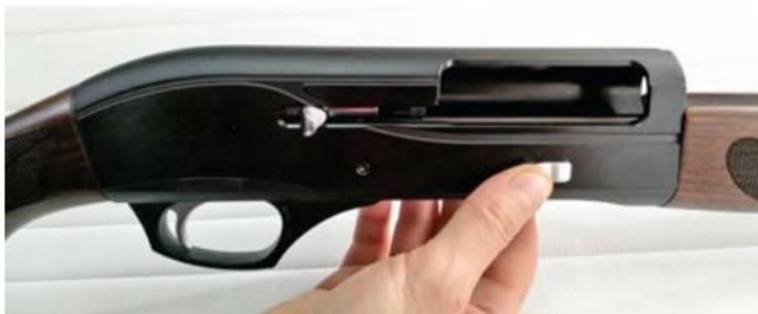
**When pressed without the barrel assembled, the bolt handle will hit the front of the ejection port and the receiver will be damaged.**
