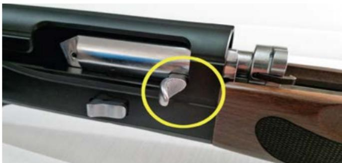
**Only for inertia (AK 212/220) wood stock models, the action bar will hit and may crack the forend before the bolt handle damages the receiver. Make sure you assemble the barrel and forend before pulling the bolt handle for cocking the action.**
